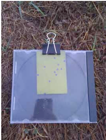
CD cases and clips secure the water-sensitive cards and keep the cards off the moist ground.
