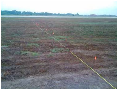
Placement of Cards illustrated to the left using a measuring tape and flags to identify interval spacing to place cards.
